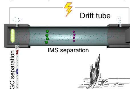
**Figure 2:** Sketch of the analyte flow in a GC-IMS
